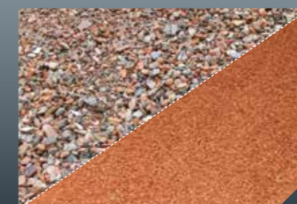
Screened C&D waste fractions
