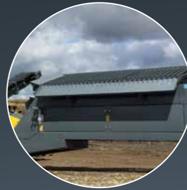
9.2 m 3 hopper, wide loading area Enables the use of wider loading buckets.
