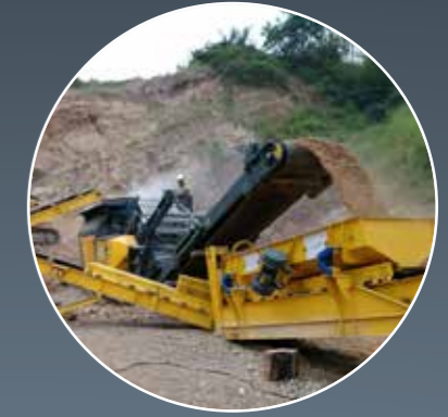
Plugs in to crusher Enormous energy savings due to screener being powered by crusher.
